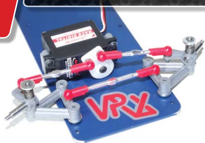
The new front-end sporting a cross brace for camber adjustments. My front arms are upside down to run smaller diameter front tyres, and I rounded off the front corners of the chassis plate
