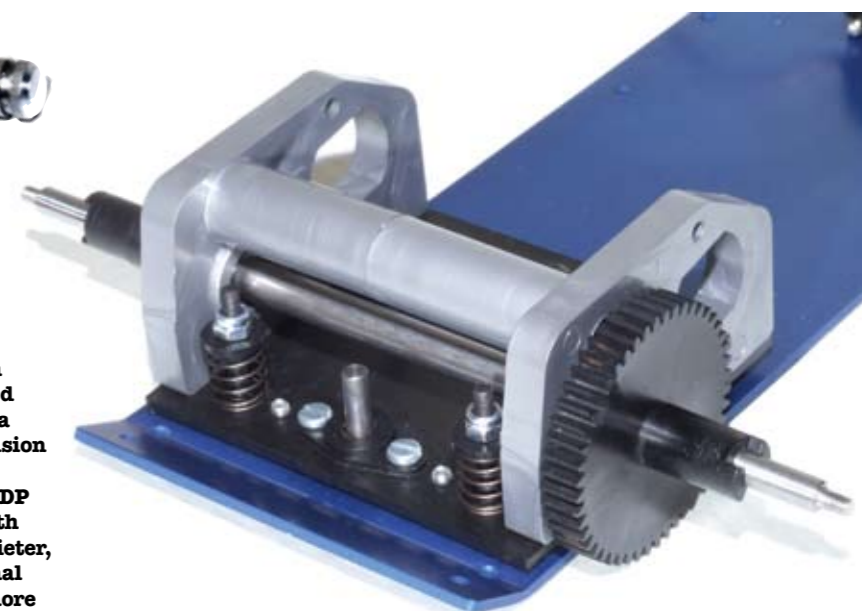
Above: Stiffer rear pod mouldings now sports droop grub screws and high speed ceramic axle bearings
